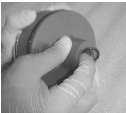
Installing PWT Seal
