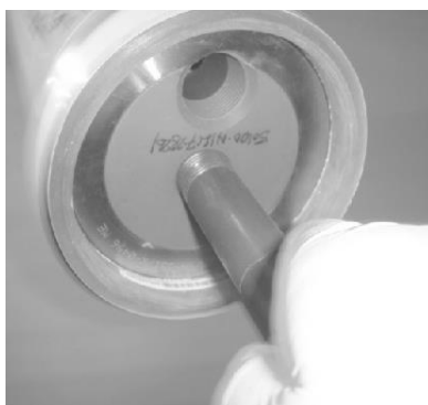
Removal of Head Assembly
