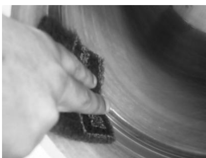
Cleaning inside the vessel
