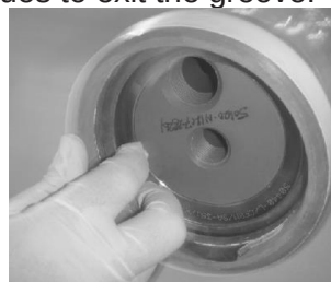
Removal of Retaining Ring
