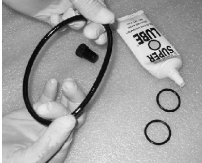
Lubricating Plug seals and O-rings
