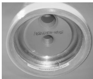
Retaining ring seated in the groove
