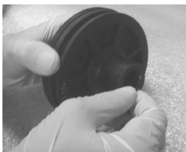
Inserting PWT seal
