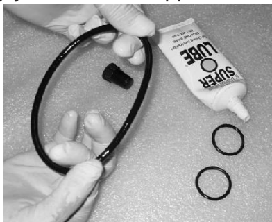
Lubricating Plug seals and O-rings
