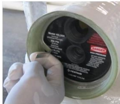
Lifting end of retaining ring out of groove
