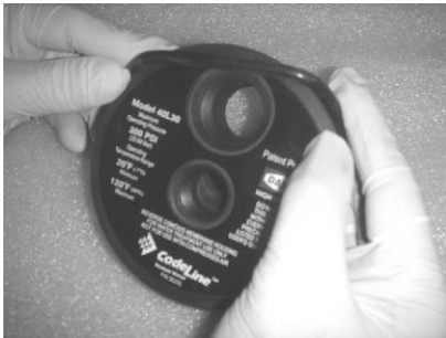
Removal of the Plug Seal
