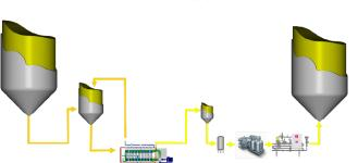
The chosen BMF-18 system was installed in the last quarter of 2011 together with an upgrade of the BBT cellar. Currently, the brewery filters beer in a high gravity process and kvass with a maximum filter capacity of up to 7000 hl per batch.
