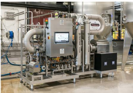
Pentair's new compact Beer Membrane Filtration (BMF) system is the ideal solution for craft and small breweries with a 10,000 to 100,000 hl annual output. The first BMF +Flux Compact S4 was installed at the Princen Brewery in the Netherlands in early 2017 and continues to operate successfully.
