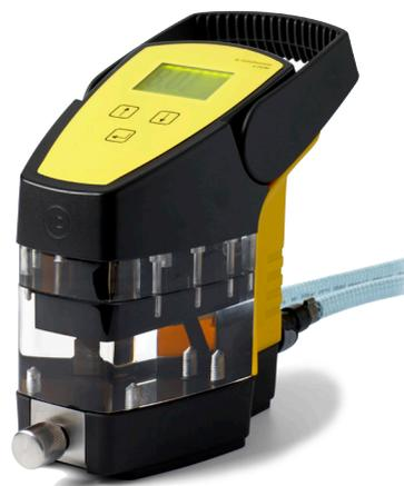
Pentair Haffmans' portable O<sub>2</sub> Gehaltemeter, type o-DGM combines high accuracy with excellent measurement stability.
