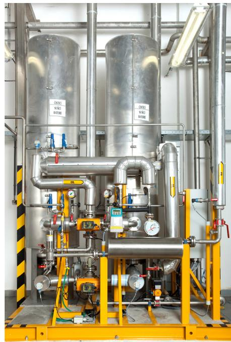
Activated Carbon Filters/Dryer
