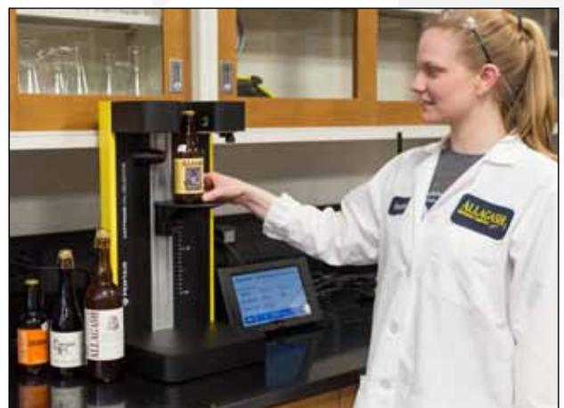
Heather Muzzy, a Quality Control Specialist at Allagash, tests the CO<sub>2</sub> level in a bottle of Allagash's signature White with Haffman's non-invasive CO<sub>2</sub>-Selector.
