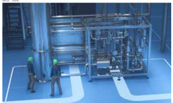
Water Deaeration System WDS
