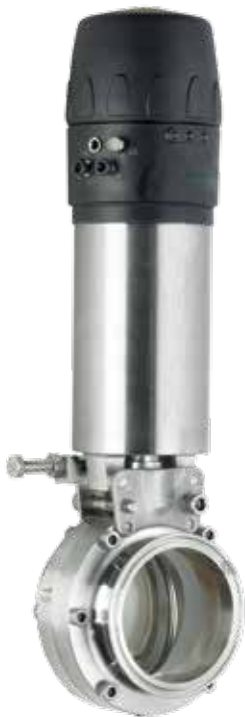
F250P/F251P Ski-Jump Butterfly Valve with Pneumatic Actuator F257 with travel stop and F783 Easymind Control Top
